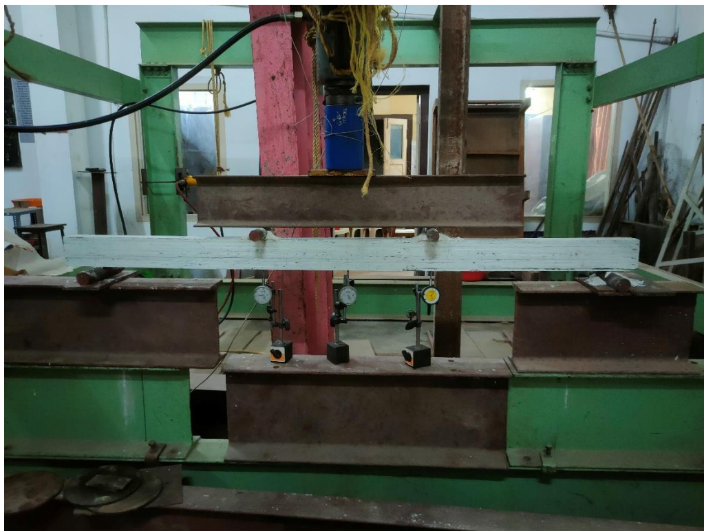
Figure 4.4: Experimental setup for beam testing
