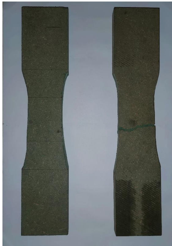
Figure 4.3: Specimen before tension test and specimen after tension test
