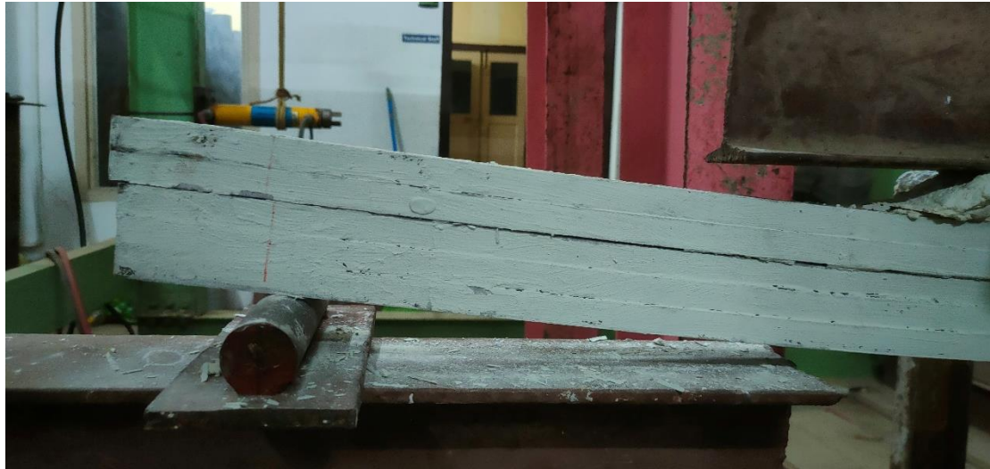
Figure 5.11: Failure due to delamination of FP specimen
