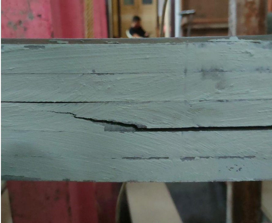
Figure 5.9: Failure due to delamination of FS specimen
