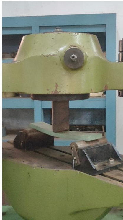
Figure 4.1: Test for modulus of elasticity and rupture
