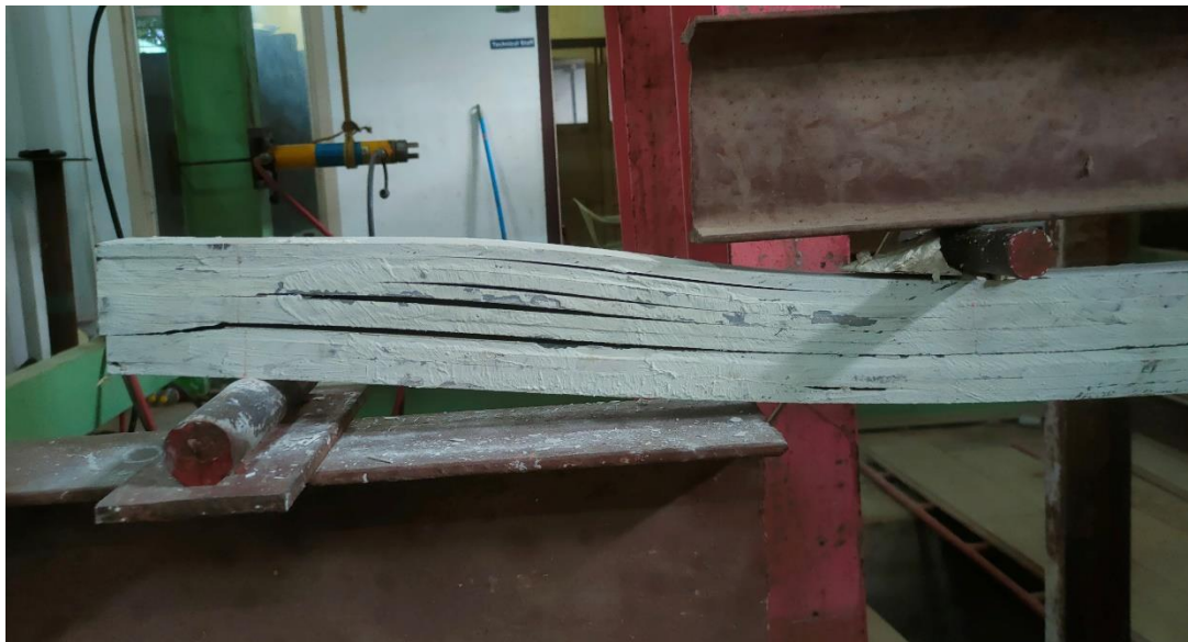
Figure 5.8: Failure due to delamination of TP specimen
