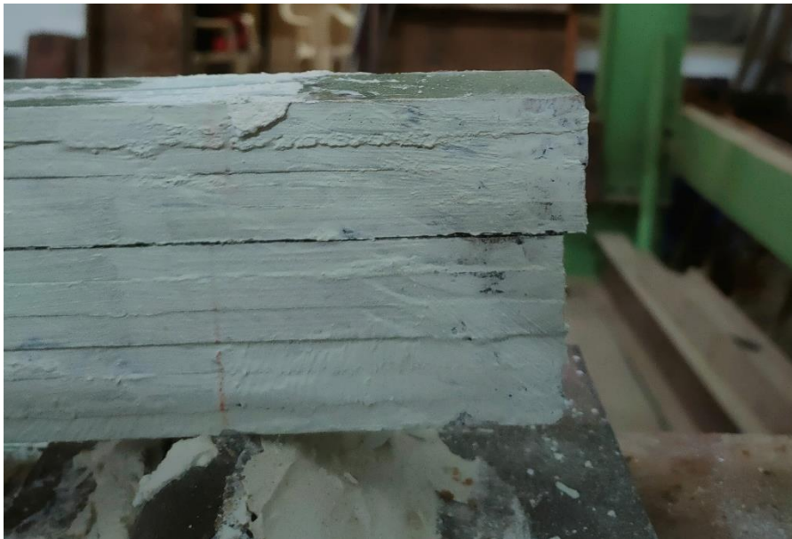
Figure 5.10: Failure due to delamination of TS specimen
