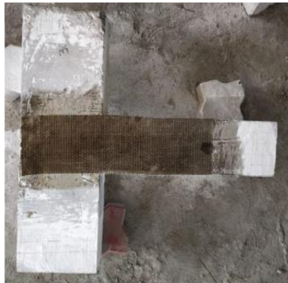
Figure 1.4 BFRP wrapping (Source: Sakthimurugan et al., 2021)
