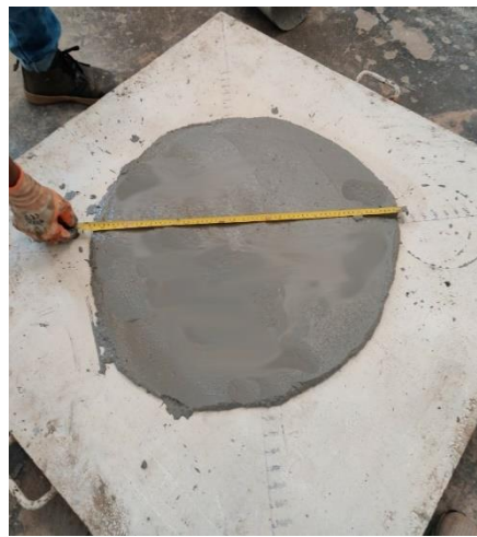
Figure 4.15 Slump flow and T 50 test
