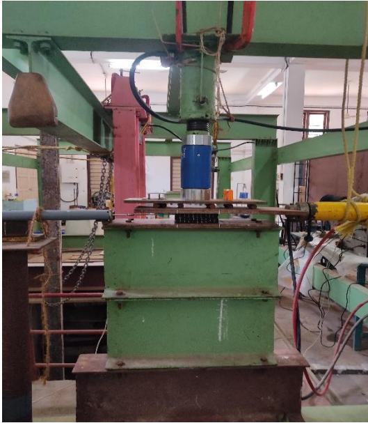
Figure 4.3. Experimental setup for cyclic loading
