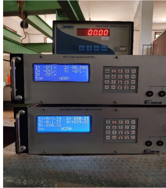
Figure 4.4. Indicators to measure the load and deformations
