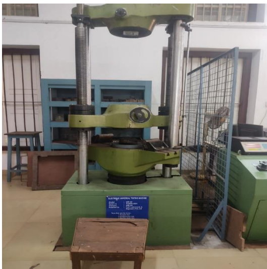
Figure 4.1 Experimental Setup for compression testing
