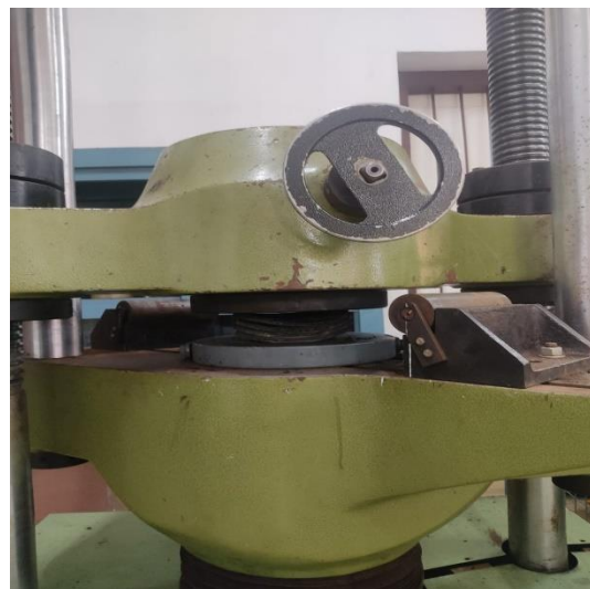
Figure 4.1. STP specimen loaded in the compression machine
