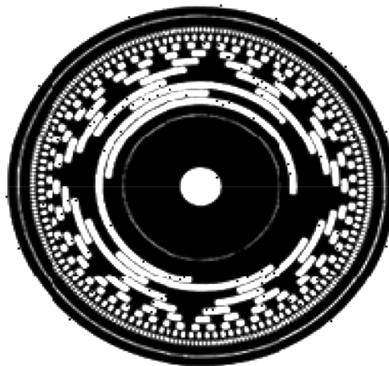
Figure 3.1: Gray coded Disk
