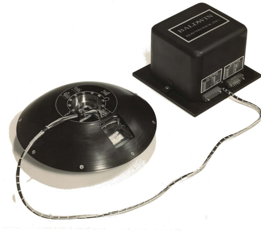
Figure 2.1: First Optical encoder used in space craft applications
