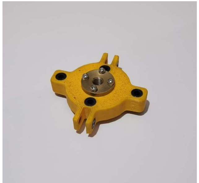
Fig 23. 3D printed Nut with bearings and brass thread insert
