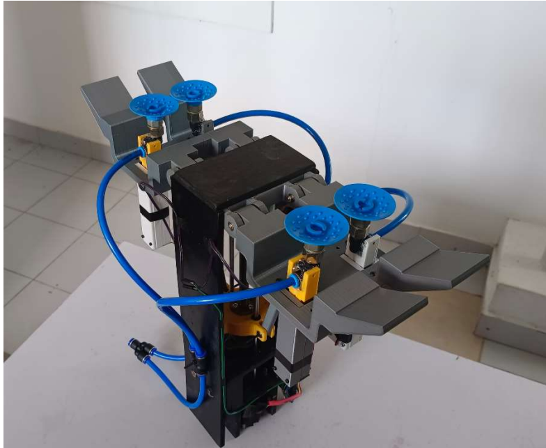
Fig 28. Finalized assembly of the end effector prototype.
