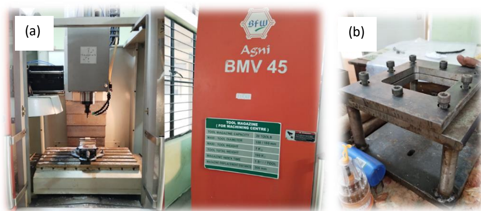
Fig.4.( a) CNC machine with forming set up
