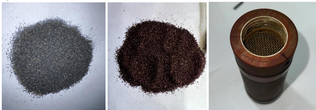
Fig:1.5 Different Regenerator Material (a) ErNi (b) HoCu2 (c) Copper Meshes (First stage)
