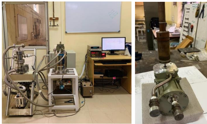
Fig 3.27. Displacers assembled on the Cam drive and the complete experimental setup
