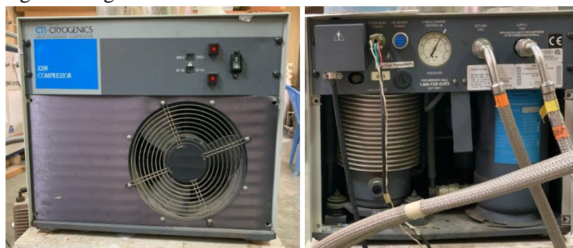
Figure:3.4 Helium Compressor
