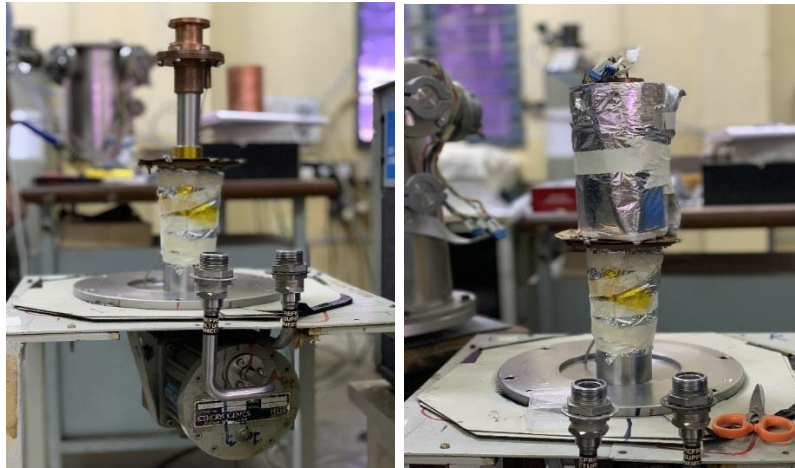
Figure 3.21: First stage insulated Figure 3.22: Second stage insulated
