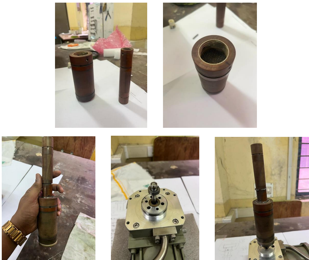
Fig.3.20 Regenerators, their housings, cam arrangement and assembly
