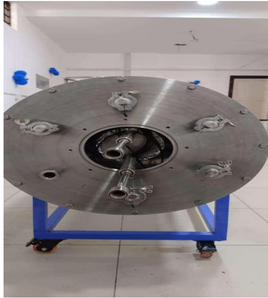
Fig.18. Flow meter with connections for capacitors with proper support in the cryostat.
