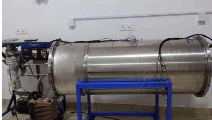
Fig 20. Cryostat connected to vacuum pump for insulating the system
