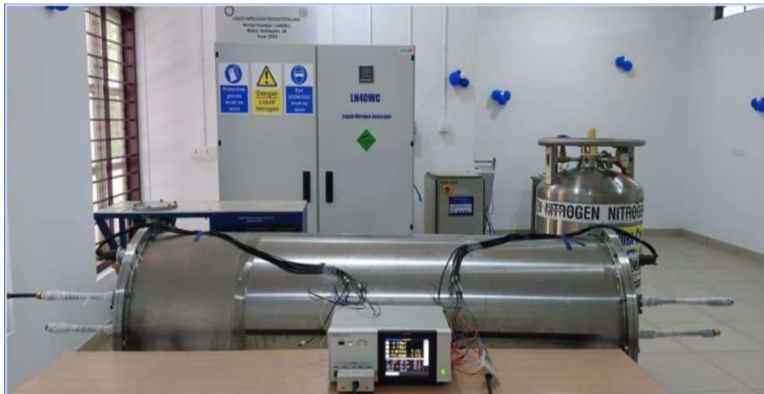
Fig 22. Experimental setup for evaluating the performance of the cryogenic flow meter
