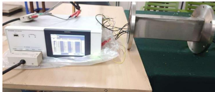
Fig.16 Testing of the capacitors using LCR meter
