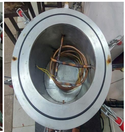
Fig.25 Brazed coil pre-cooling setup
