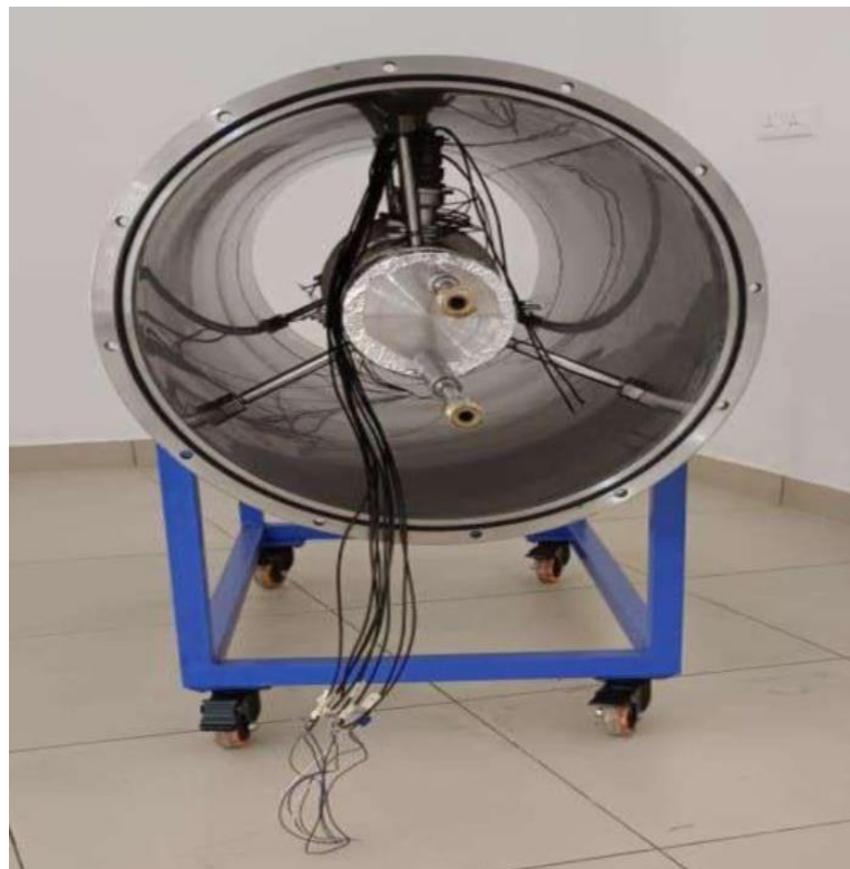
Fig.17 Flow meter with connections for capacitors
